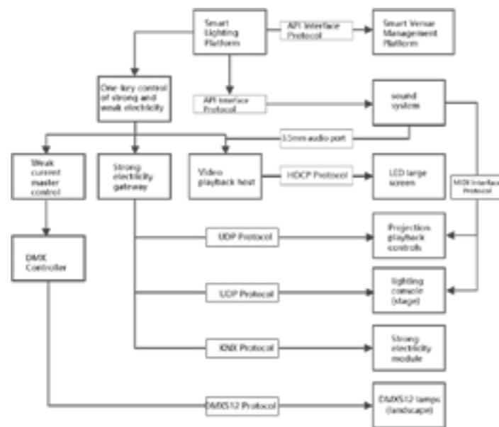
Figure 3 Communication protocol of smart lighting control system
