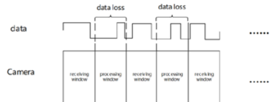
Figure 3 Synchronization protocol reception processing process
