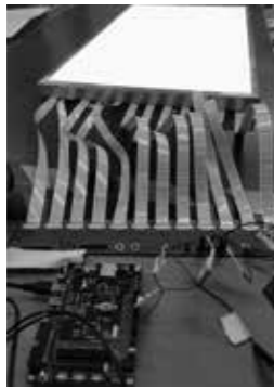
The FPGA for AM IC to drive white light Mini-COB backlight module.
