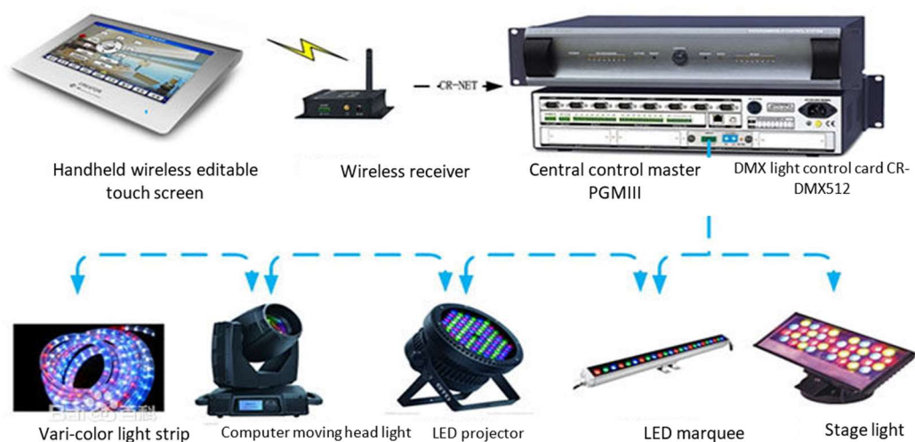
Figure 4 Schematic diagram of DMX512 control system
