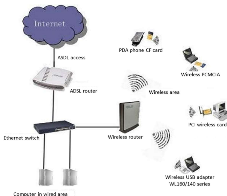
Figure 10 Schematic diagram of Wi-Fi network
