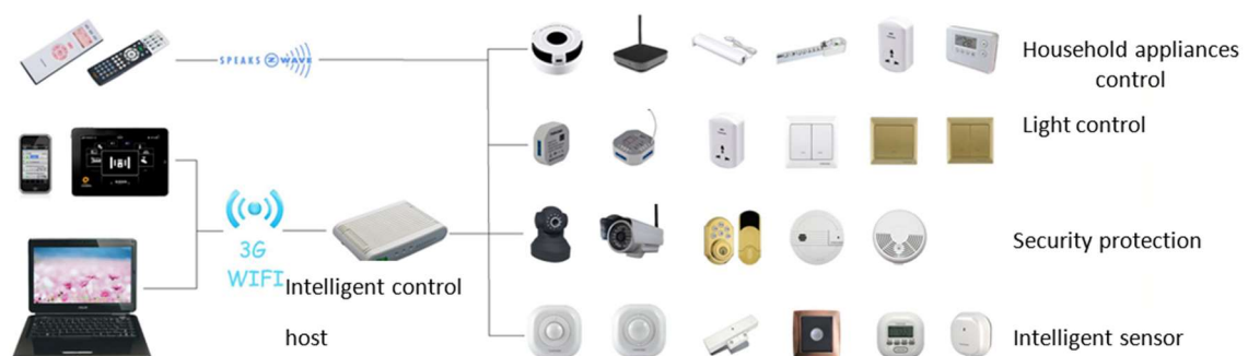
Figure 16 Schematic diagram of Z-Wave control system
